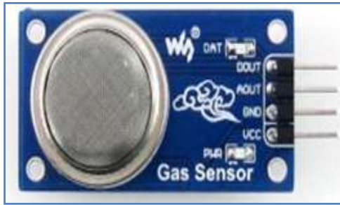
Fig. 4 (a) Front view of MQ-135 Gas Sensor
